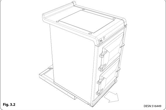
2. Position the plinth alongside the AGA eR7 leaving no gap between the two plinths (Fig. 3.3).
